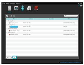
3 Select a streaming service and click the **□** button at the bottom. The **Setup – Streaming Service** window appears. Select the **Information** tab
