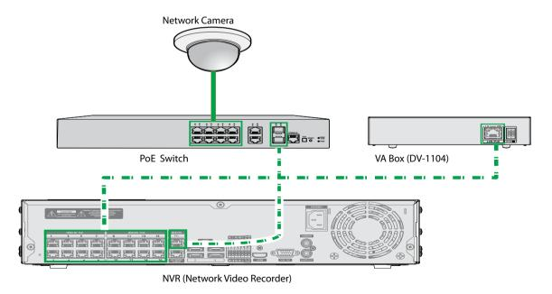
Example 3: VA Box Connection Diagram Using PoE Switch
