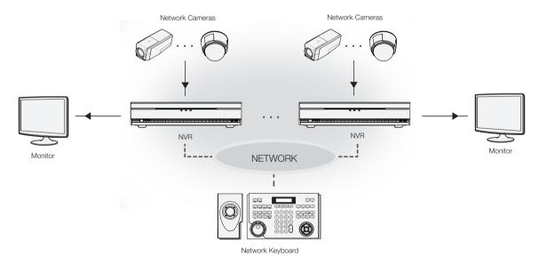
You can control NVRs and PTZ cameras connected to the NVRs via a network. For more information, see Part 2 - Installation > NVR System Registration and Part 3 - Operations > Controls for NVR System.
