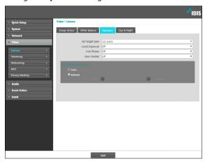
AE Target Gain: Specify exposure compensation's target gain. Exposure is compensated automatically based on the specified target gain. Higher the gain, brighter the images.
