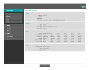
Quick Setup allows you to set up **System**, **Network**, **Video**, **Audio**, and other basic settings needed for camera use.
