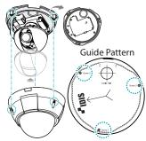
1 Use the screws provided with the camera to secure the bottom cover on a wall or a ceiling.
