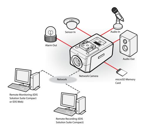
Control the camera over the network from software installed on a computer. Ideal for using the camera over the network from a remote location.
