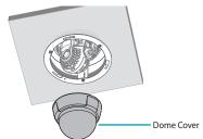
5 Assemble the bracket lid to the bracket.
