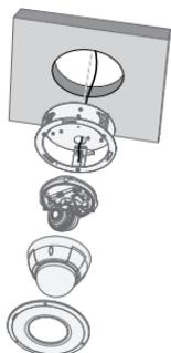
This manual is intended for the users of the FM1200 ceiling mounting bracket. It includes the instructions for mounting the FM1200 ceiling mounting bracket to the ceiling.
