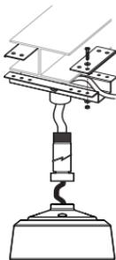
This manual is intended for users of the DA-CM1400 ceiling mounting bracket. It includes instructions for mounting the DA-CM1400 ceiling mounting bracket to an I-beam.
