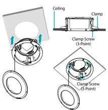
3 Connect the network cable and the power adapter. Attach the camera to the install mount. Turn the camera clockwise to fasten.
